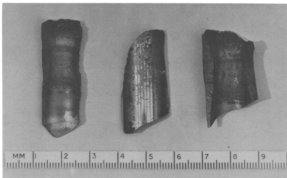
Figure 2 Samples of compact indium phosphide prepared by the reaction of indium monochloride and phosphine.
